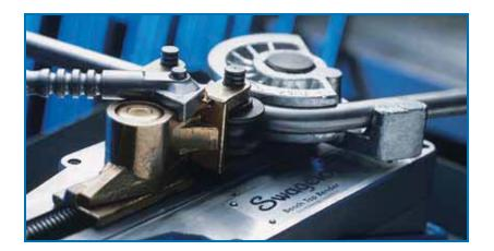
Swagelok tube benders make routing easier. They bend tubing to any angle up to 180 degrees. 45 and 90 degree fittings are replaced by tubing bent exactly as you need it. Routing can be more precise. Offsets and odd angles are no longer a problem. The flow improves and space is conserved.
