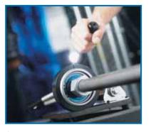
Preswage the Swagelok nut and ferrules onto the tube using the multihead hydraulic swaging unit;
